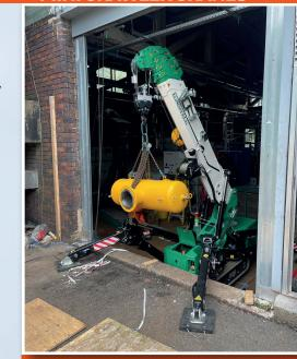
The angles and orientations of the crane's outriggers can be adjusted to suit the site
