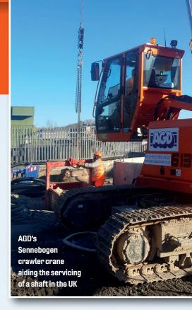
The counterweight, previously located externally on the rear of the crane, is now built in the frame to eliminate the space occupied by the rotating turret at the back of the machine.
